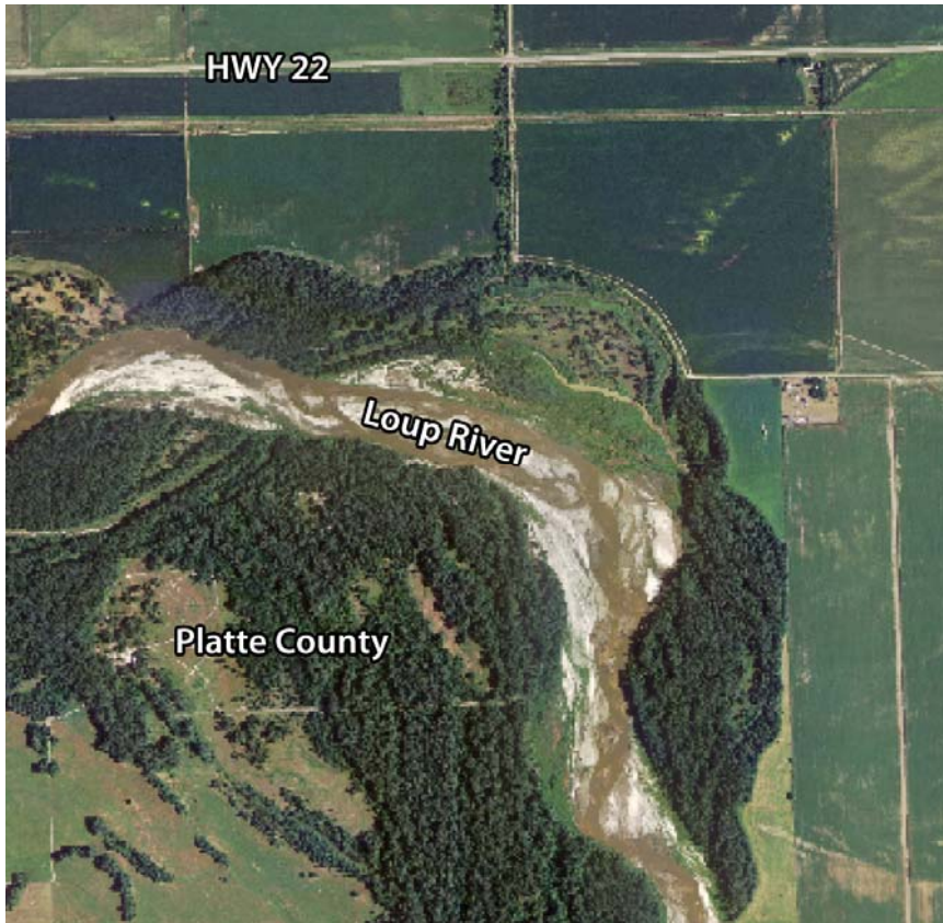
Photo 5-3. Aerial view of the Loup River, south of Nebraska State Highway 22 in Platte County, showing meandering and braided characteristics.
